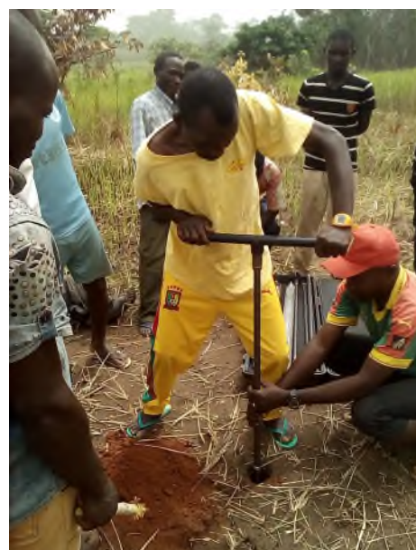
Photo 2: Artisanal Mines in SCED-Ndelengue, practicing the use of the hand augers. Photo by Hervé Pounou.
