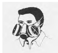
Mask: To protect the nose and mouth. Not recommended for spraying.
