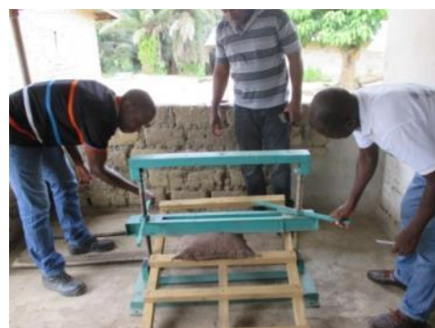
Figure 4: Cassava press being tested for defects by USAID FED's equipment technician at Wainsue, Bong County
