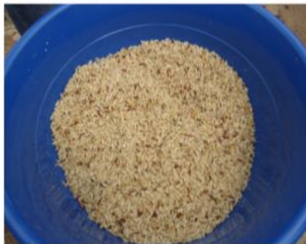
Photo 7: Parboiled rice milled by impact rice dehuller (95% grain and 5% paddy)
