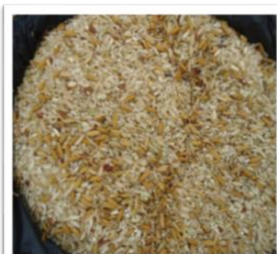
Photo 6: Un-parboiled rice milled by impact rice dehuller (40% grain and 60% paddy)
