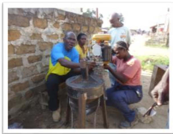
Photo 1: Fixing and testing of the impact rice dehuller
