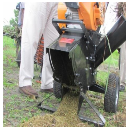
Figure 9: Compost shredder breaks down material for fast efficient compost production.
