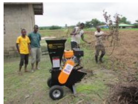
Figure 35: Compost shredder breaks down material for fast efficient compost production.
