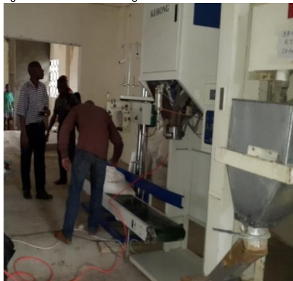
Figure 7: The new rice milling line installed at FABRAR Liberia's industrial processing plant in Kakata
