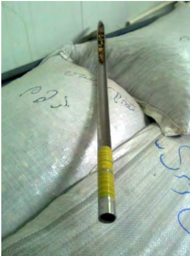
Inshell probe. Note, notations of grower on sack.
