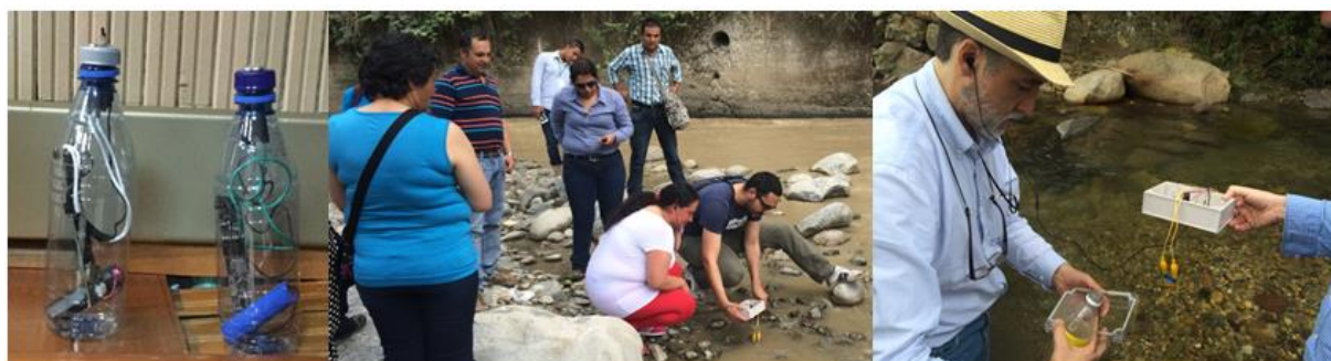
Left: Riffle water sensor developed by Public Lab that measures conductivity and temperature. Center and right: Probe to determine water quality in advanced stage of its development. The probe measures water quality through readings of conductivity, dissolved oxygen, temperature, and pH.
